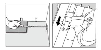
**Cutting tip:** If cutting with a jigsaw, the floor surface should be turned down. Otherwise always cut with the floorboard facing up.
