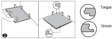
First row, second tile: Insert the end tongue on the short side of the second tile into the end groove of the first one and rotate downward to assemble. Make sure both tiles are perfectly aligned.
