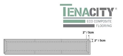
Set saw depth to the board's overall thickness. Cut along lines and remove the center section.
