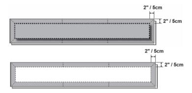
Cut along lines to make relief cuts, then carefully lift and pull center-length cuts first using a chisel, then work into corners to remove end pieces last.
