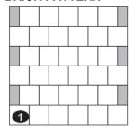
Begin laying in the left-hand corner, with the grooved edge visible and facing outward. Use spacers between the wall and the floorboard in order to keep a 10 mm gap.
