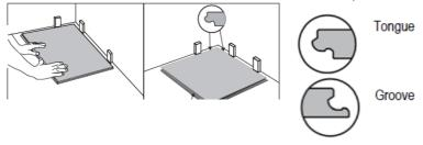
1. First row, second tile: Insert the end tongue on the short side of the second tile into the end groove of the first one and rotate downward to assemble. Make sure both tiles are perfectly aligned.
