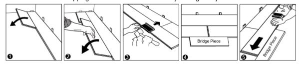
**Tip**: After finishing the installation of every row, use a tapping block or a cutoff and a rubber mallet to gently tap the tiles into the click of the previous row to make sure they are tightly clicked together and make sure there is no gap between the long side of the tiles installed. Any gapping can compromise the whole installation.
