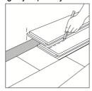
4. **Holes for pipes:** Measure the diameter of the pipe and drill a hole that is 20 mm larger. Saw off a piece as shown in the figure and lay the board in place on the floor. Then lay the sawed-off piece in place.
