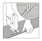
5. Door molding and skirting: Lay a board (with the decorative side down) next to the door molding and saw as shown in the figure. Then slide the floorboard under the molding.
