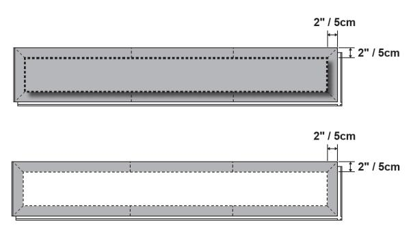
• Cut along lines to make relief cuts, then carefully lift and pull center length cuts first using a chisel, then work into corners to remove end pieces last.
